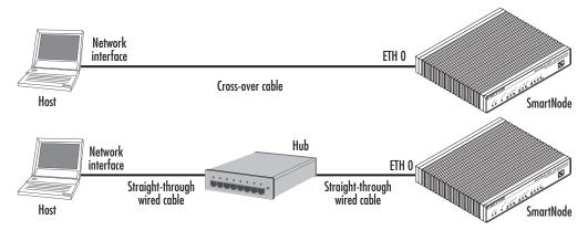
Figure 3. Connecting the SmartNode to the network
